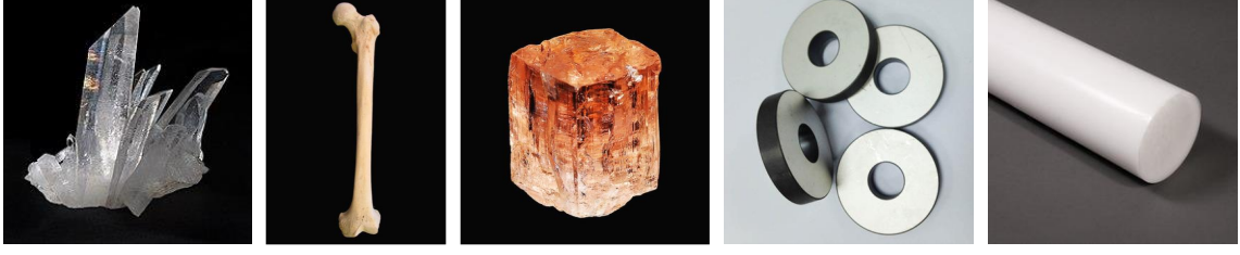
Figure 2.3: Natural piezoelectrics: Quartz, human bone, and topaz. Synthetic: PZT ( Lead Zirconate Titanate ) and PVDF ( Polyvinylidene Fluoride ), respectively.
