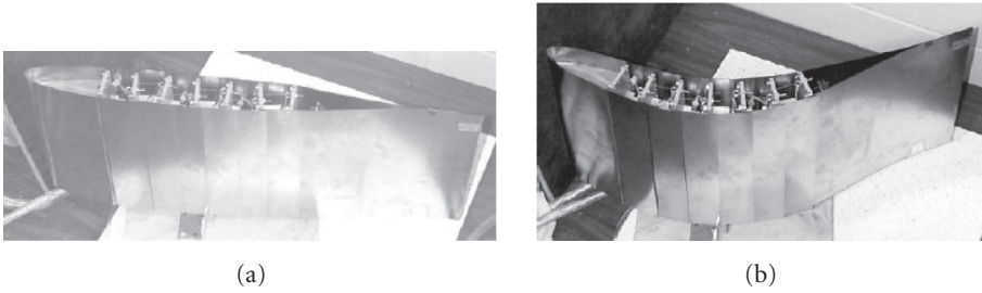
Figure 3.1. SMA multiactuated hydrofoil prototype (Rediniotis et al. [60]).
