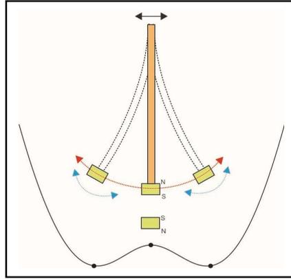
Figure 1. Schematic bistable piezomagnetoelastic system.
