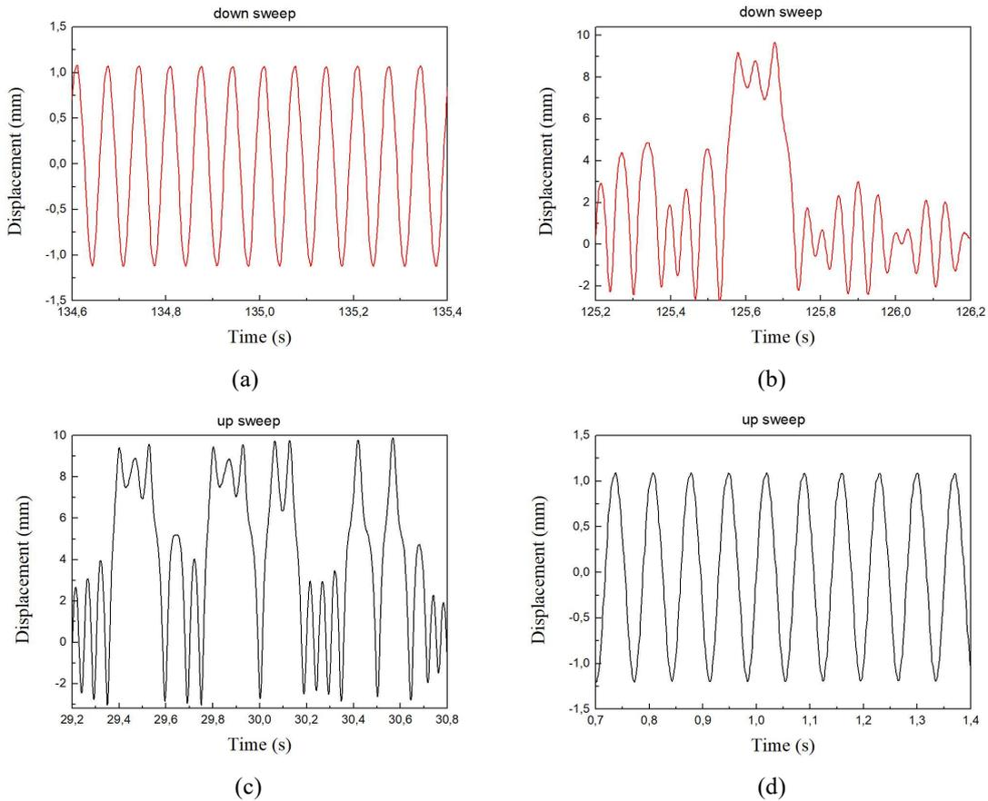
Figure 5. Experimental result of signal behavior. (a) 15 Hz (b) 17 Hz (c) 20 Hz (d) 26 Hz
