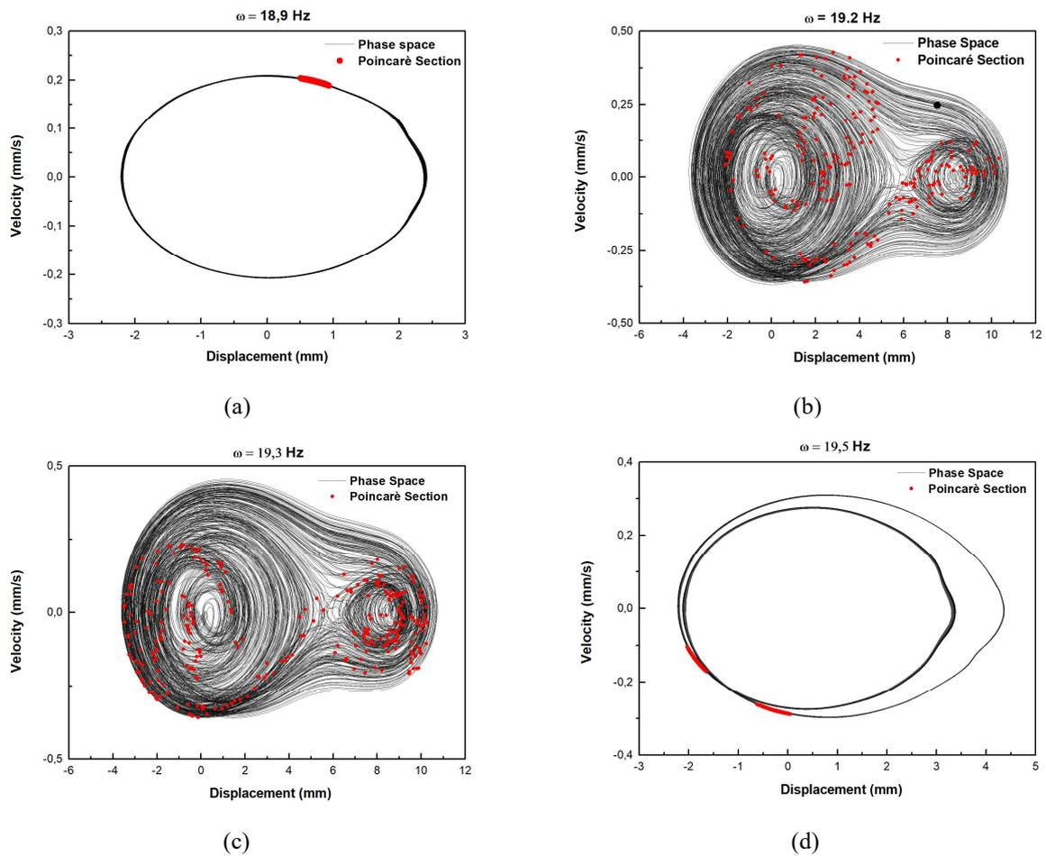
Figure 7. Phases space and Poincaré Section for: (a) 18.8 Hz – Period-1 response, (b) 19.0 Hz – Chaotic-like response, (c) 19.4 Hz – Chaotic-like response, and (d) 19.7 Hz – Period-2 response.
