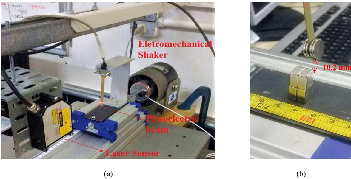
Figure 3. Experimental Apparatus. Sensors setup (a) and nonlinear configurations (b).
